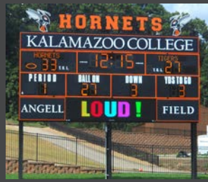
32' Football Scoreboard with Electronic Team Names (ETN) and a 16'x4' Full-Color Message Center
